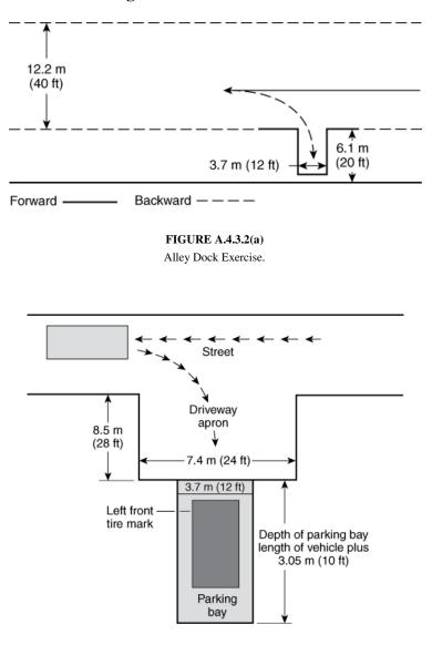
FIGURE A.4.3.2(b) Station Parking Procedure Drill. (A) Requisite Knowledge. Vehicle dimensions, turning characteristics, spotter signaling, and principles of safe vehicle operation.
